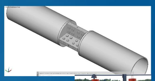
Our modular design ensured that the parts are easily bolted together with no welding on the construction site.
