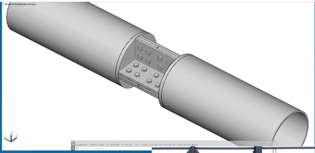
Our modular design ensured that the parts are easily bolted together with no welding on the construction site.
